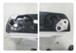
12. Disassemble the Door S/W with tools. Be careful not to scratch.
